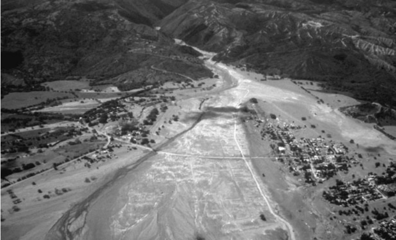
FIGURE 1 This view across what remained of the town of Armero, Colombia, shows the devastation caused by volcanic mudflows in November 1985. The massive mudflows were generated by an eruption of Nevado del Ruiz, 30 miles away. The flows followed the Lagunillas River and then burst out onto the floodplain from the canyon visible at the head of the alluvial fan near the top of the photo. The 131-foot-high mudflows overwhelmed the town, and 23,000 residents died in the catastrophe. (Photo: US Geological Survey's Volcano Disaster Assistance Team)
